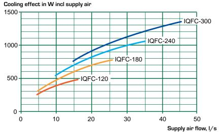
The diagram shows the approximate cooling effect P<sub>tot</sub> in W with water flow q<sub>w</sub> = 0,05 l/s, temperature difference between room air and supply air  $\Delta t$ = 8 °C, pressure drop 60 Pa on the air side and max. sound pressure level LA10 = 30 dB(A).
